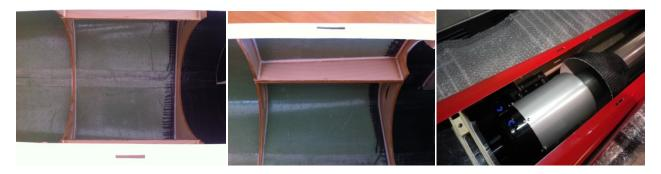
Fixed with epoxy glue the tank air support for landing gear under the Kevlar tank.
